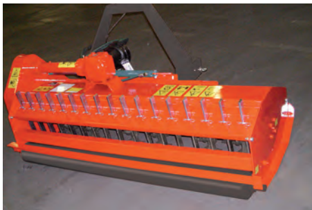
The Kubota SE3000 series can be equipped with rake tines to improve chopping on prunings.
